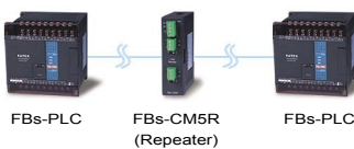
The RS485 repeater FBS-CM5R can be used to extend the distance and expand the range of RS485 network
